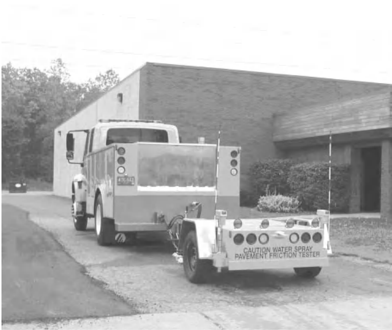
Figure 9.41 Friction Tester (Courtesy of Dynatest Inc.)
