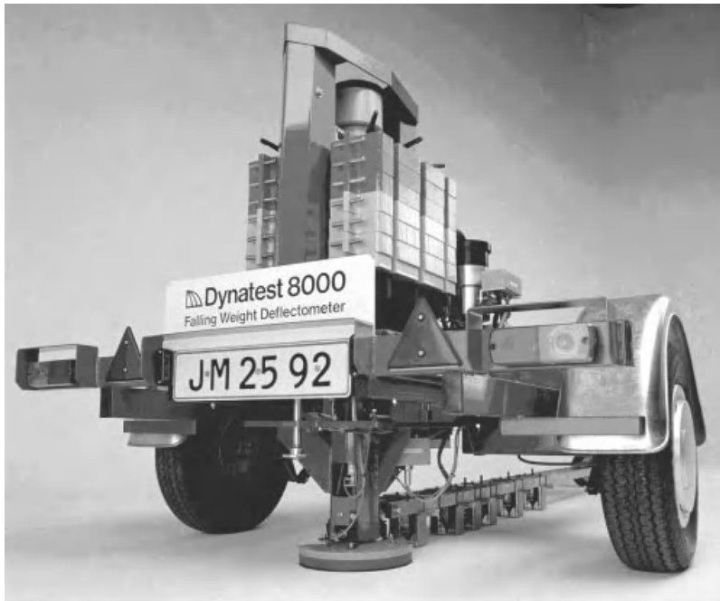
Figure 9.26 A Falling Weight Deflectometer (Courtesy of Dynatest Inc.)
