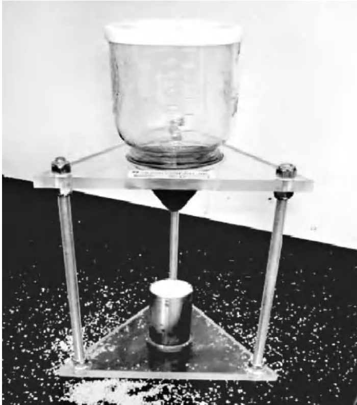
Figure 4.6 Uncompacted Void Content of Fine Aggregate Apparatus. Courtesy of FHWA
