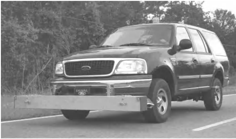
Figure 9.13 Modern High-Speed Profilometer. (Courtesy of Dynatest Inc.)
