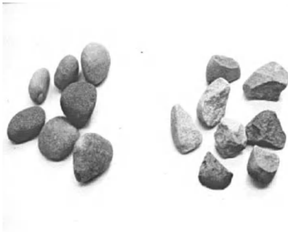
Figure 4.8 Illustration of Counting Percent of Fractured Faces. Image courtesy of Gilson, Inc.
