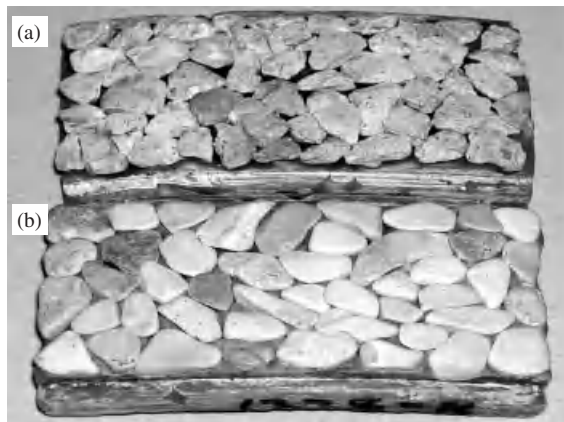
Figure 4.16 Aggregate Coupons (a) before Polishing and (b) after Polishing Using the British Wheel.
